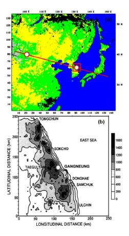
Fig. 1:Topographical features in (a) the vicinity of Korean peninsula for numerical simulation using WRF-2.2 model and (b) the mountainous coastal region surrounding Gangneung city (20 m above mean sea level) and Mt. Taegulyang (860 m) in a fine-mesh domain (horizontal resolution of 3km). In (a), circles denote Gobi Desert and Gangneung city.
